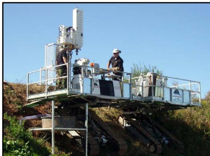
All of the rigs (with the exception of hand held) are capable of carrying out SPTs and CPTs and taking 70mm diameter samples. We can also install a range of instruments in the boreholes including inclinometers, extensometers, standpipes and piezometers (BAT, VW and standard).
